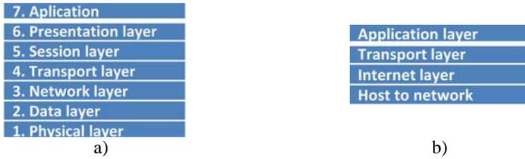
**Figure 2:** a) Layers of the ISO-OSI model. b) TCP/IP Internet protocol layered model.
